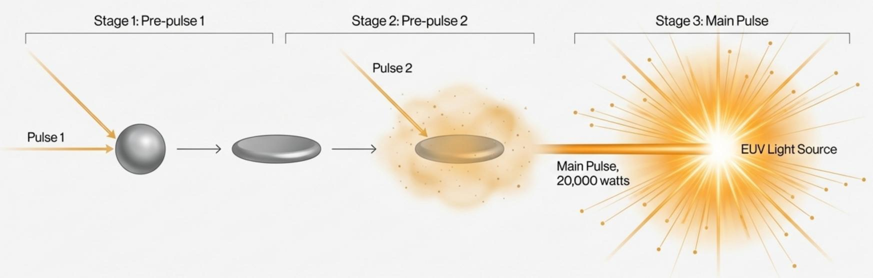
This multi-pulse process creates tiny supernovas inside the machine, 50,000 times a second.
