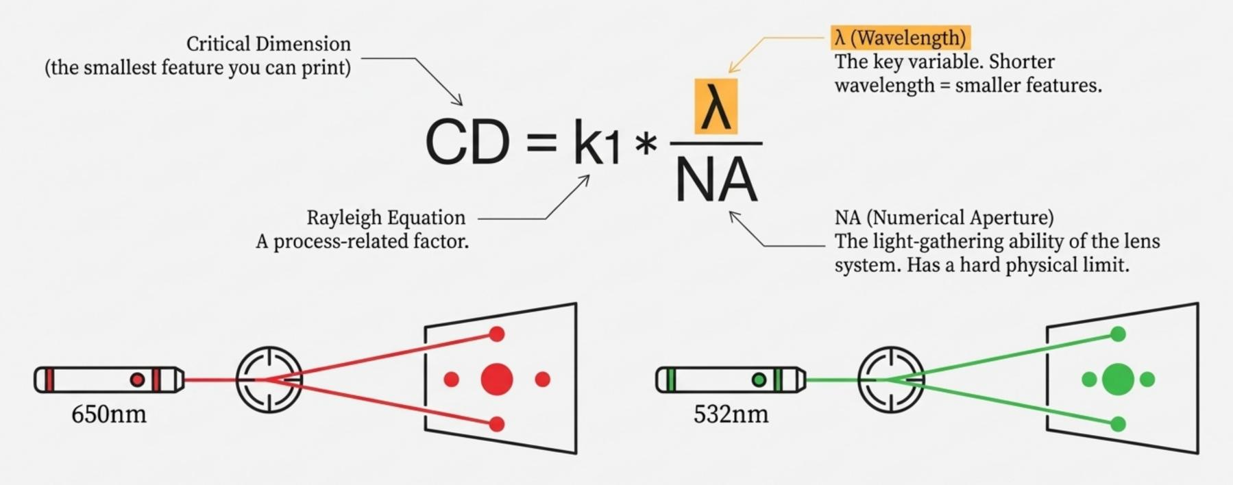
To keep shrinking features, the industry had to use shorter and shorter wavelengths. By the late 1990s, they were stuck at 193nm Deep UV (DUV) light, and Moore's Law was about to hit a brick wall.
